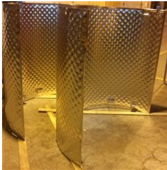
Manufactured hydroformed components of the PPC thermal shields
